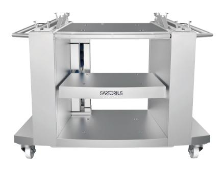
The FlexAct® BT is equipped with two plate holders, each of them consisting of two metal plates with porous spacer between which single-use bags are inserted for inflation and integrity testing. By using porous spacers, the film surface of the bag is not in direct contact with the stainless-steel holder during the test. Any potential masking effect is eliminated. The masking effect will occur when a leak in the plastic film is pressed against a smooth surface, blocking the leak.
